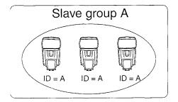
For example, if you have the slave ID set to  $< \mathbf{A} >$  for three Speedlites, all three Speedlites will be controlled as if they were one Speedlite in slave group A.
