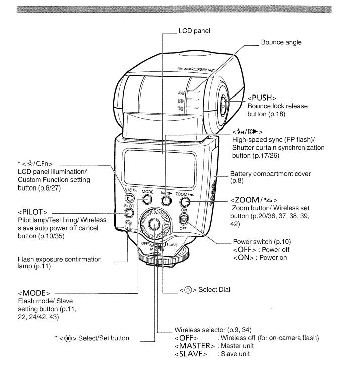
Asterisked buttons have a timer that keep the button's function active for 8 sec. (⊘8) after you let go of the button. The <☆ > illumination lasts for 12 sec.
