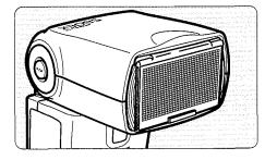
Pull out the wide panel and place it over the flash head as shown. The flash coverage will then be extended to 14mm.
