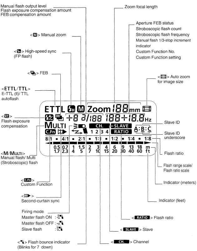
• To illuminate the LCD panel, press the  $< \frac{1}{2}$  > button.
