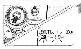
Press the <<>> button so that the <>> icon and flash exposure compensation amount blink.
