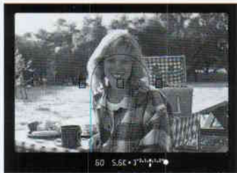
Partial metering circle
