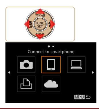
8. Press the < A > < V > buttons to choose [Add a Device], and then press the <FUNC./SET> (@) button.
