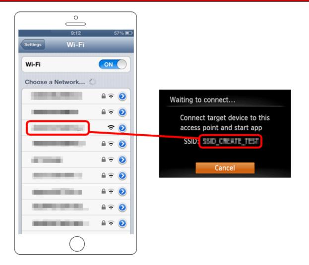
For better security, you can require password input by accessing MENU and choosing [ **11**] tab > [Wi-Fi Settings] > [Password] > [On]. In this case, enter the password displayed on the camera in the password field on the iPhone when it is displayed.
