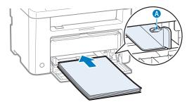
4 Adjust the paper guides tightly to the width and length of the paper.
