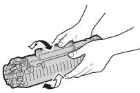
3 Insert the toner cartridge, close the upper unit, and then lower the operation panel.
