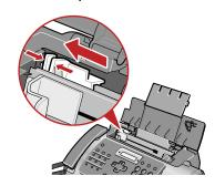
3 Tap the edge of the stack on a flat surface to even the stack.
