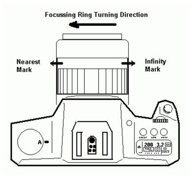
tiny further movement of the focusing ring after you get the indicator might induce a significant off-focus result. Hence it is good to practise well a technique of stop turning the focusing ring once the indicator shines.
