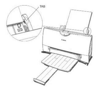
Make sure there are no gaps between the stack of paper and the paper guide nor the right edge of the sheet feeder.
