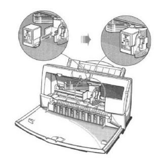
Press the lock lever down completely; do not use excessive force.
