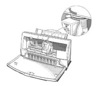
o If you installed the BC-21 Color BJ Cartridge, set the paper thickness lever to the center.
