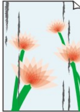
Printed Surface Is Smudged
