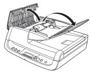
Raise the roller unit's lock lever. (Gently bend the lock lever inward, then raise it.)
