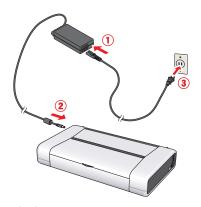
Do NOT connect the USB cable at this stage.
