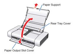
The Paper Output Slot Cover will open automatically.
