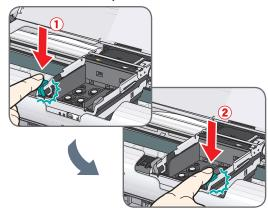
Make sure that the Print Head Lock Lever is firmly locked into the Print Head Holder by pressing both tabs on the Print Head Lock Lever until it clicks.
