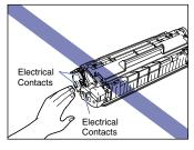
• Whenever you are handling the toner cartridge, hold it as shown in the diagram, and keep the surface marked with the arrow facing up. Do not stand it on its end, or turn it upside down.
