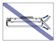
• Keep pulling on the tape until it is fully removed from the cartridge. If any sealing tape is left inside the toner cartridge, you may experience printing problems.
