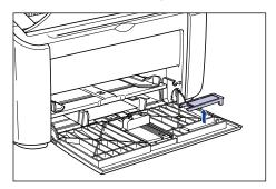
☐ Insert the small paper guide from directly above, as shown in the diagram, then fold it towards the back.
