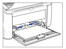
2 Load the envelope with the printing surface facing up and the flaps closed and on the left side, then gently insert them all the way to the back of the tray.
