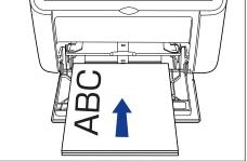
4 Slide the paper guides to fit both sides of the stack.
