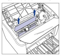
$\hfill \square$  If the jam is difficult to clear, pull the paper out from the multi-purpose tray or manual feed tray.
