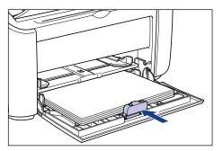
If the paper jam occurred while feeding from the manual feed tray, load paper into the manual feed tray.
