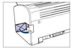
3 Connect the B-type (square) end of the USB cable to the USB connector on the rear side of the printer, and close the USB cover.
