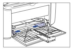
3 Load the envelopes with the printing surface facing up and the flaps closed and on the left side, then gently insert them all the way to the back of the tray.
