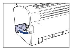
Connect the B-type (square) end of the USB cable to the USB connector on the rear side of the printer, and close the USB cover.
