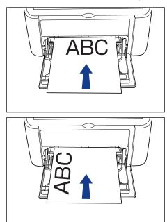
3 Slide the paper guides to fit both sides of the stack.
