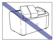
• If you try to close the multi-purpose tray while the rear paper guide is sticking out of the tray, you may damage the printer. Always check to make sure that rear paper guide is pushed all the way back into the multi-purpose tray before you close the multi-purpose tray.
