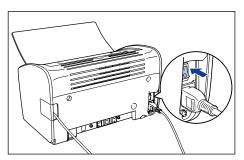
The printer Power Indicator turns on and the printer runs a self-diagnostic test. If there are no errors in the self-diagnostic test, the printer is ready to print.
