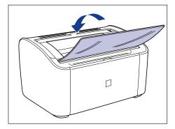
6 Grasp the left and right side of the printer with your hands, as shown in the diagram, and firmly hold onto the printer when you carry it.
