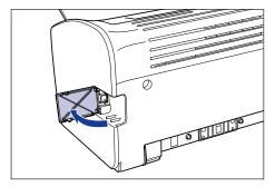
3 Connect the B-type (square) end of the USB cable to the USB connector on the rear side of the printer, and close the USB cover.
