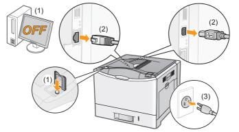
When installing or removing the optional accessories, be sure to turn the printer OFF, unplug the power plug, and then disconnect all the interface cables and power cord from the printer. Otherwise, the power cord or interface cables may be damaged, resulting in a fire or electrical shock.
