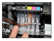
Please make sure that every cartridge is well installed according to the color label.
