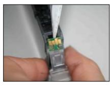
Pay attention when you remove original chips. Make sure that the chips are not damaged.
