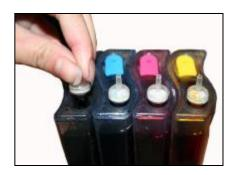
Put the Air-filter into the Air-hole
