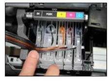
Then put the CISS cartridges into printer
