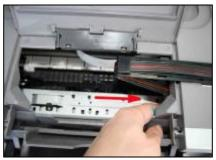
Please make sure there will be no block and collision when the cartridges move from one side to the other.
