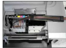
Clip the tube into the support arm as the pictures shown.
