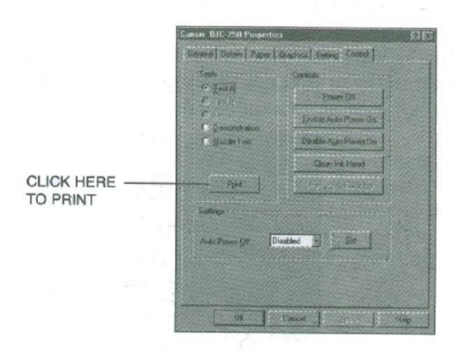
Before selecting a Tests option, make sure paper is properly loaded in the sheet feeder (see *Automatically Feeding Paper* starting on page 3-7).
