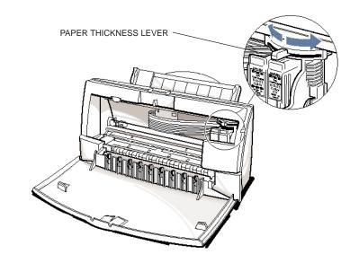
Be sure to check this lever when you change BJ cartridges, and before and after printing on heavier-weight print media or envelopes.
