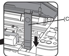
Lift the Scanning Unit (Cover) (B) until it locks into place.
