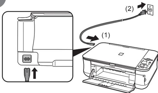
Plug in the power cord on the left side of the machine and connect the other end to the wall outlet.
