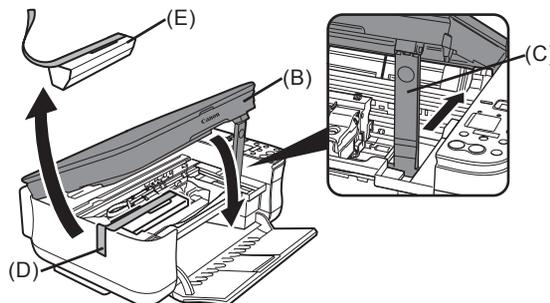
Pull the orange protective tape (D) and remove the protective material (E).
