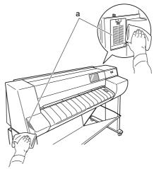
4 Plug the power cord into the power source.
