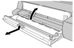
7 Lower the roll release lever toward the inside of the machine, release the paper guide, then pull out the left and right corners of the leading edge of the media as far as the roll so the media is parallel with the sides and even with the roll.
