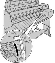
**3** If the W7250 is used without the optional stand, open the tray then the roll media tray and manually turn the roll holder to take-up the roll media until it is away from the paper guide.
