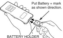
Install battery and Battery Holder into Remote Control Unit.
