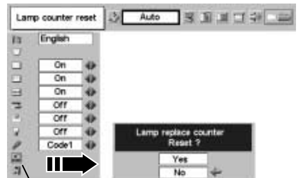
Move the pointer to Lamp counter reset and then press SET button. The message "Lamp replace counter reset?" is displayed.
