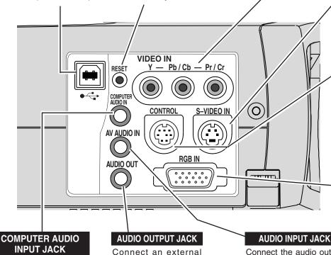
Connect the audio output (stereo) from the computer to this jack. (Refer to P12.) Connect an external audio amplifier to this jack. (Refer to P12, 13.) Connect the audio output from your video equipment to this jack. (Refer to P13.)
