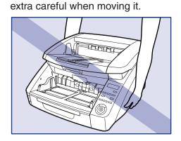
☐ When lifting up the scanner, make sure you do not grasp the knob on the Document Feed Tray on the front of the scanner.
