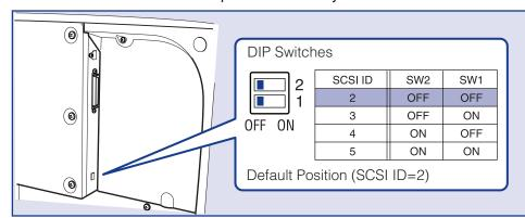
• The scanner incorporates a SCSI terminator which is permanently set to ON. When using a daisy-chain configuration with other SCSI devices, make sure that the scanner is connected as the last device in the chain. Set the terminators of all other devices to OFF.
