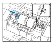
6. Pull the roller lock lever down to lock the retard roller in place.
