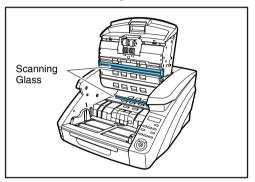
5. Wipe the rollers using a moistened and firmly wrungout cloth while rotating the rollers.
