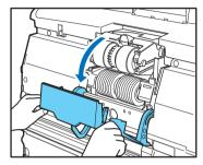
3. Pull the roller lock lever down.
