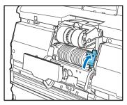
Close the roller cover. Make sure to hear a latching sound and that it is securely returned to its original position.
