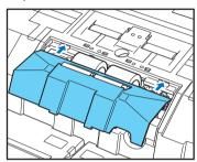
2. Push the front of the retard roller cover in. Make sure to hear a latching sound that it is securely returned to its original position.
