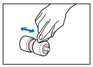
8. Wipe away the dirt from the pad mounted to the retard roller cover while removed using a cloth that has been dipped in water and thoroughly wrung.
