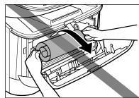
Do not pull the jammed paper upward.
