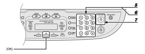
**5** Enter the destination name (max. 20 characters, including spaces) with the numeric keys, then press [OK].
