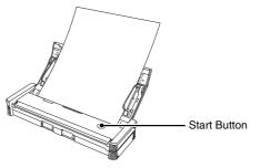
If you load the document in the scanner and press the Start button, CaptureOnTouch starts and scanning starts according to the settings of the assigned job.
