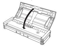
The scanner turns OFF, and the power indicator goes out.
