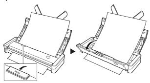
**3** Remove the jammed document from the feed side or eject side.
