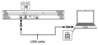
If necessary, connect the power supply USB cable.
