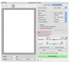
If you select the [Check the image of the first page] check box, only one page of the document is scanned and the corresponding scanned image is displayed in the preview window.
