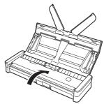
After you remove the jammed paper, check to see if the last page was scanned correctly, and then continue scanning.
