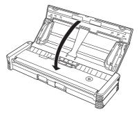
**3** Push the section (front cover) at the front of the feed tray to close it.
