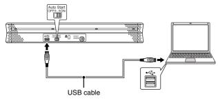
If necessary, connect the power supply USB cable.
