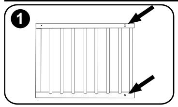
1. Loosen screws on gate (2X).
