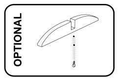
To permanently attach foot to gate, attach with screw.
