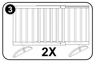
3. Slip feet onto bottom of gate.
