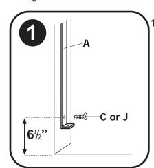
Install hinge bracket (A) to wall (stationary side of gate) using Phillips screw (C) beginning 6½" above floor surface. (Use ruler on left edge of this sheet to measure from floor).
