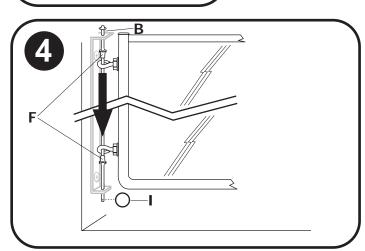
Hang gate by inserting hinge rod  $(\mathbf{B})$ , through top of mounted hinge bracket  $(\mathbf{A})$ , through upper plastic 4. shoulder washer (F), through both eye bolts, through lower plastic shoulder washer (F), and finally through bottom of hinge bracket. To sécure hingé, insert key ring (I) through hole in end of hinge rod.
