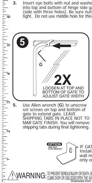
5. Use Allen wrench (G) to unscrew set screws on top and bottom of gate to extend gate. LEAVE SHIPPING TABS IN PLACE NOT TO MAR GATE FINISH. You will remove shipping tabs during final tightening.
