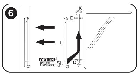
Mount latch assembly (K) to gate using 3/4" bolts with serrated washers (**D**). Attach wall mount for latch assembly (**H**) up into part (**K**) that is now secure on gate. Slide gate out to mark holes for (**K**) on attaching wall. (\*OPTIONAL ONE WAY BRACKET INSTALLED HERE) Then attach the wall mount of latch assembly to wall using Phillips head screws (C).
