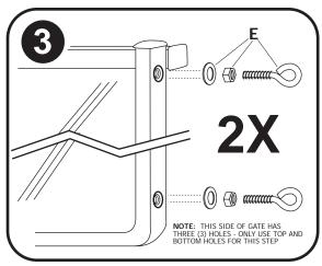
3. Insert eye bolts with nut and washer (E) into top and bottom of hinge side gate (side with three holes). Be sure nuts are tight. Do not use middle hole for this step.
