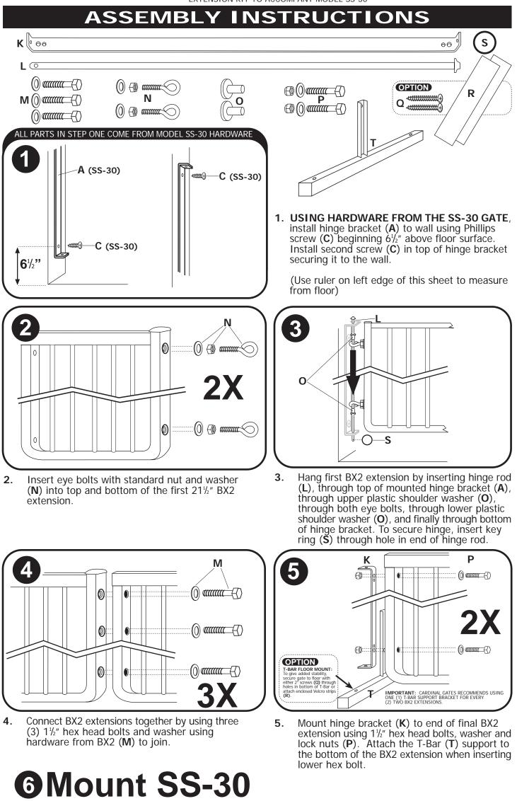
the Stairway Special gate to hinge bracket (K) that was mounted in **STEP FIVE**.
