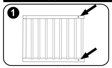
Loosen screws on gate (2X).
