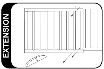
If you have purchased an extension, attach with two (2) bolts and nuts through top and bottom of extension to current gate. Next add single foot to added extenstion.
