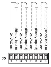
The terminals for Inputs 3, 5, and 8 are available for use in place of the flying wire leads at Molex connectors **J1** and **J2** identified below:
