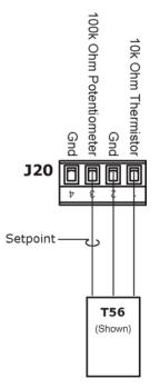
**NOTE J20** Analog Inputs 10 and 11 are reserved for a 10k Ohm space temperature sensor with an optional 100k Ohm offset potentiometer used for setpoint adjustment.
