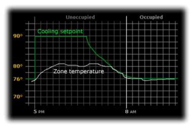
The actual equation that the controller uses to calculate **Optimal Start** is nonlinear. An approximation of the result is shown below.
