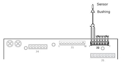
NOTE Sensor termination requires installation of RTU Open wiring harness assembly (Part #OPN-RTUHRN).
