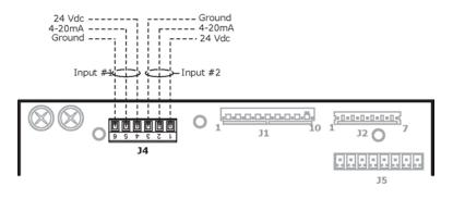
**NOTE J4** Analog Inputs 1 and 2 may be set for the following device types:
