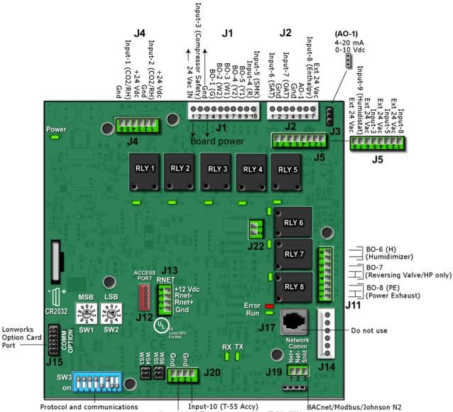
baud rate selector DIP switches
