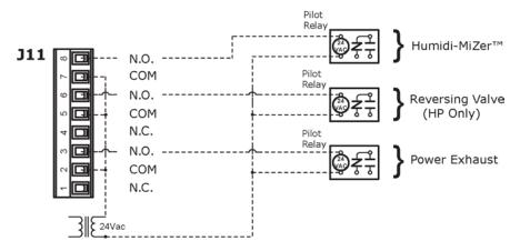
**NOTE** Output relay contacts rated at 3A, 24V maximum. Install pilot relays required by application.
