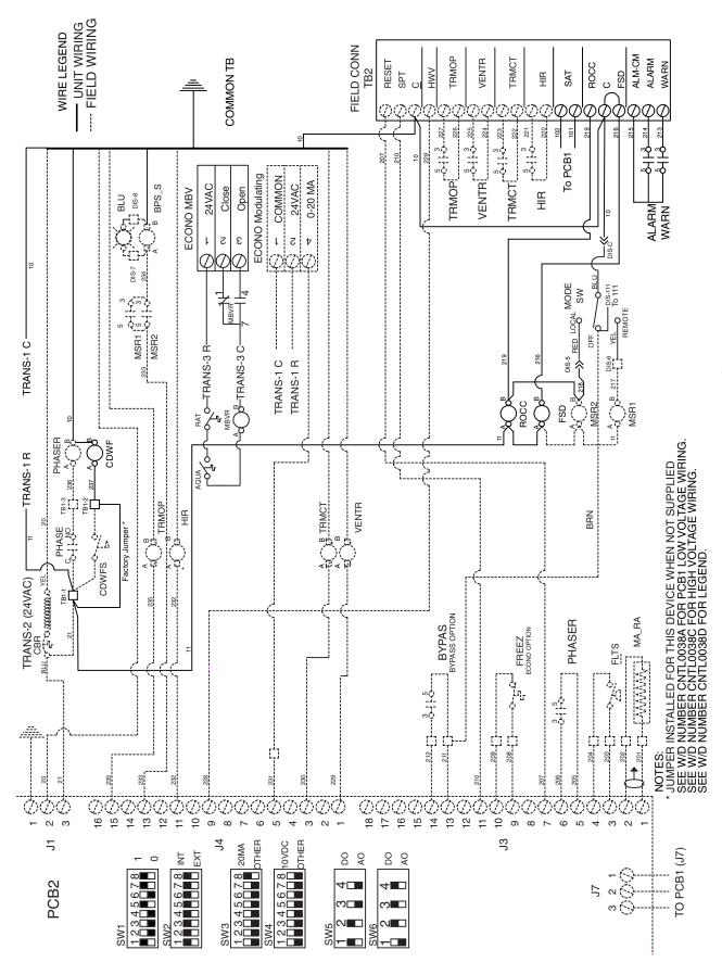
50BVJ,K,W,X Field-Installed Low Voltage Schematic
