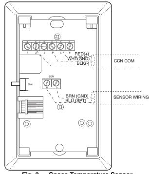
Fig. 3 — Space Temperature Sensor Typical Wiring (33ZCT55SPT)
