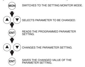
Fig. 8 — 50BV VFD Display Function Keys
