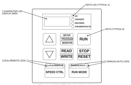
Fig. 6 — 50XJ VFD Display Keypad
