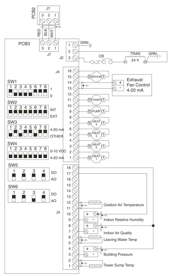
50BV,XJ Accessory Control Module (PCB3) Schematic
