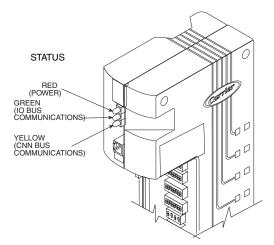
Fig. 1 — CC6400 Control Module LEDs
