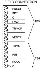
Fig. 2A — Field Terminal Blocks for 50XJ Unit
