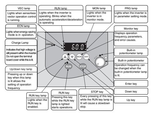
Fig. 7 — 50BV VFD Display
