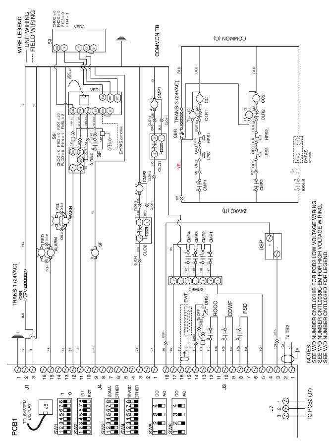
50BVJ,K Field-Installed Low Voltage Schemtic
