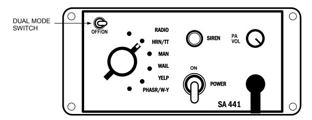
The Toggle Power Switch controls the siren power. The siren may be left on any time the vehicle is in operation. The power should be turned off when vehicle is not being used to conserve battery power.
