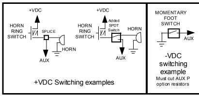
**Cutout Input Connection** - The Cutout Input turns off any siren tone output when activated, and remains off until a control is activated or changed. The adjacent diagram shows two connection examples. See the INSTALLER-SELECTABLE OPTIONS section for programming details.
