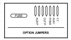
**Auxiliary Input Function** - The auxiliary input normally activates the Horn function. Do not cut the jumper resistor labeled "AUX I".
