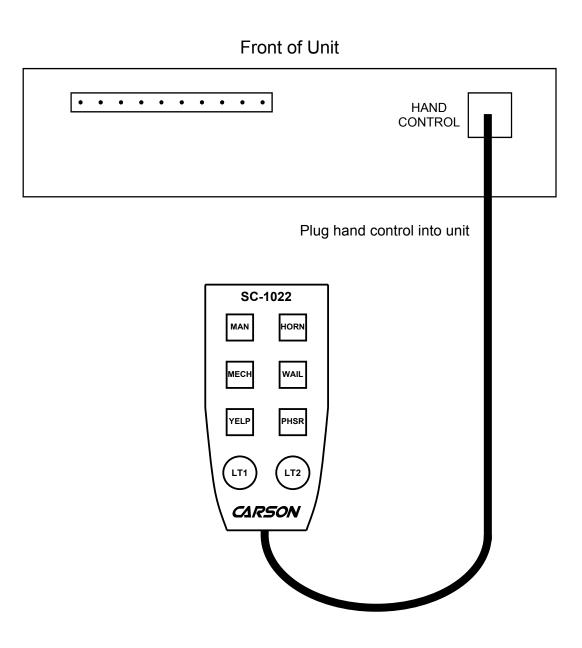
Note: Cable may be extended with ED1753 Hand Control Cable Extension Kit.
