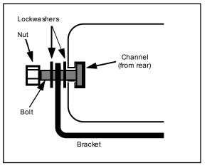
**SC-1012 Remote Panel**: The remote panel of the SC-1012 is typically mounted underneath the vehicle dashboard using mounting hardware. Mount the panel in a location away from the driver's or passenger's legs.
