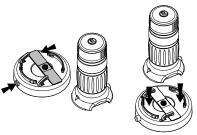
Secure the zPix to the Specimen Stage and connect the USB Cable (7) to a USB port on your computer.\* The LED light will turn on indicating the the device is powered on. Insert the CD and follow the prompts to start up the Digital Viewer<sup>TM.</sup> Software.
