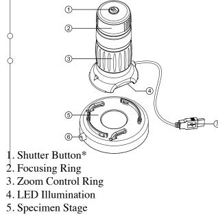
6. Specimen Slide Releasing Button7. USB Cable
