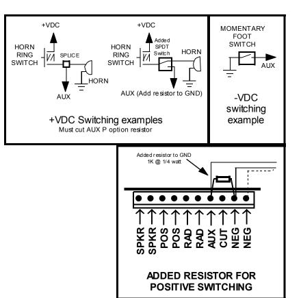
**Cutout Input Connection** - The Cutout Input turns off any siren tone output when activated, and remains off until a control is activated or changed. The adjacent diagram shows two connection examples. See the INSTALLER-SELECTABLE OPTIONS section for programming details.
