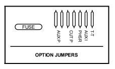
**Auxiliary Input Function** - The auxiliary input normally activates the Horn function. To activate the Man/Phsr function with the auxiliary input cut the jumper resistor labeled "AUX I".
