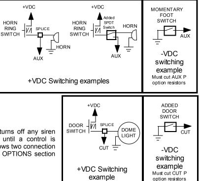
**Cutout Input Connection** - The Cutout Input turns off any siren tone output when activated, and remains off until a control is activated or changed. The adjacent diagram shows two connection examples. See the INSTALLER-SELECTABLE OPTIONS section for programming details.
