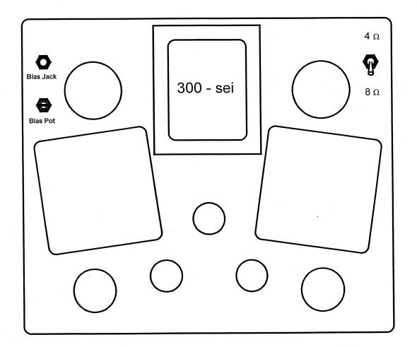
Insert the meter plug into the bias jack. Adjust for 150 mA to 160mA reading on volt ohm meter or DC current meter. Readjust the setting after the amp has warmed up for 10 minutes. Remove the bias adjustment plug and enjoy the music!
