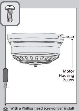
With a Phillips head screwdriver, install the four motor housing screws found in the hardware bag. Tighten all four screws securely.
