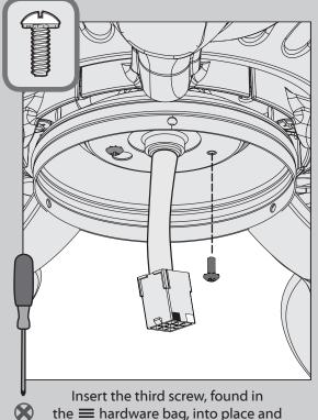
the  $\equiv$  hardware bag, into place and then tighten all three screws.
