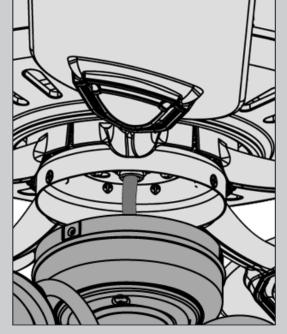
Lift the lower switch housing up until the holes line up with the screw holes in the upper switch housing.
