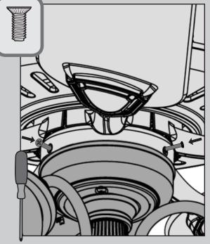
Solution Insert three switch housing screws found in the  $\equiv$  hardware bag.
