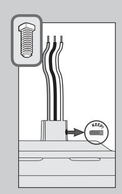
Remove the pre-installed setscrew so that the downrod can be inserted.
