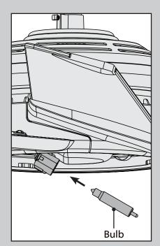
Install a halogen bulb in the light socket. When necessary, replace with bulbs of the same type and wattage.
