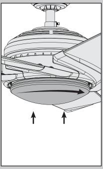
Carefully lift the globe up inside the light kit as far as it will go, then rotate the globe clockwise until it is held tightly in place by the four tabs.
