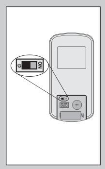
If a light kit is installed on your fan, choose the light bulb mode by moving the toggle switch. For halogen bulbs, set the switch to "ON." Replace the battery door.
