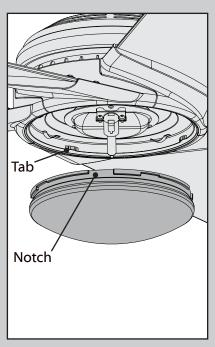
Position the notches in the outer rim of the globe so they line up with the tabs on the inside of the rim on the light kit.
