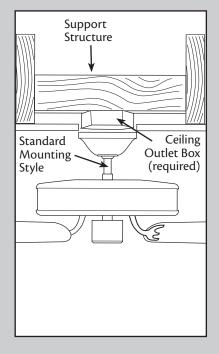
Use **Standard Mounting** or **Low-Profile Mounting** to hang the fan from a flat ceiling.
