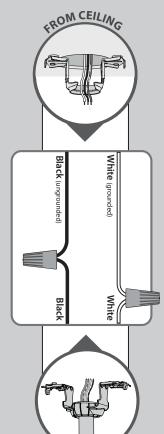
Using orange wire connectors from the 🖈 hardware bag, connect the black wire (ungrounded) from the ceiling to the black wire from the fan. Connect the white wire (grounded) from the ceiling to the white wire from the fan.
