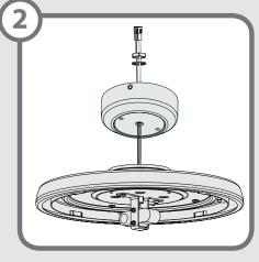
Feed the wires through the center hole in the switch housing, the washer, and the nut. Install the switch housing by twisting clockwise onto the threaded rod. Install the washer and nut onto threaded rod and tighten securely.
