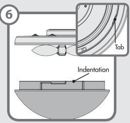
Installing the globe (sold separately)-Position the indentations in the outer rim of the globe so that they line up with the tabs on the inside surface of the light fixture rim. Carefully lift the globe up inside the light fixture as far as it will go. Rotate the globe in a clockwise direction until it is held tightly in place by the four tabs.
