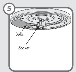
**Installing the bulbs** - Install a bulb into each of the sockets. When necessary, replace with bulbs of same type and wattage.
