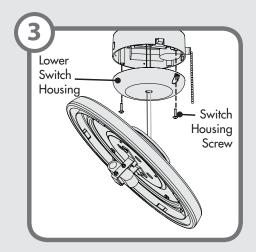
Lift the lower switch housing up so that the screw holes line up with the holes in the upper switch housing. Install the switch housing screws and tighten securely.
