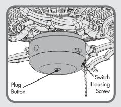
If your fan's switch housing cap resembles this one, remove the whole switch housing by removing the switch housing screws with a Phillips head screwdriver. Remove the plug button using a standard screwdriver. Then follow the **TYPE-C ASSEMBLY INSTRUCTIONS** on pages 8-9.
