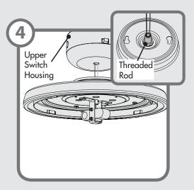
Lift the light kit up, tucking the wires into the hole in the switch housing. Install the center stem of the light kit into the lower switch housing by turning the threaded rod clockwise into the threaded hole. Continue turning until tight.
