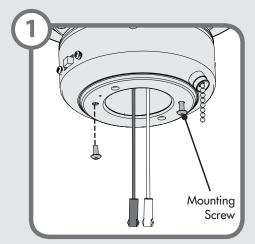
Partially install the two mounting screws into the bottom of the lower switch housing.
