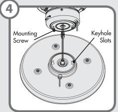
Lift the light kit up to meet the lower switch housing. Wrap keyhole slots around the screws and twist counterclockwise. Tighten screws.
