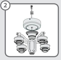
Feed the wires through the center hole in the switch housing, the washer, and the nut. Push the center hole in the gasket over the threaded rod of the light kit. Then install the switch housing by twisting clockwise onto the threaded rod. Install the washer and nut onto threaded rod and tighten securely.
