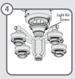
Lift the light kit up to meet the lower switch housing. Align the light kit screws with the threaded holes in the lower switch housing. Tighten screws securely.
