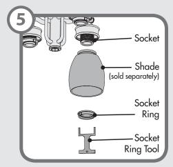
Installing the shades (sold separately)-Remove the socket rings from the sockets. Install each shade onto a socket. Install the socket rings onto the sockets by turning them clockwise using the socket ring tool.
