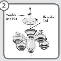
Feed the wires through the switch housing cap, washer, and nut. Then install the switch housing cap by twisting clockwise onto the threaded rod, making sure the gasket stays in line with the top of the light kit. Install the washer and nut onto threaded rod and tighten securely.
