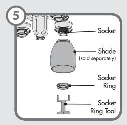
Installing the shades (sold separately)-Remove the socket rings from the sockets. Install each shade onto a socket. Install the socket rings onto the sockets by turning them clockwise using the socket ring tool.
