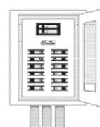
Circuit Breaker or Fuse Box
