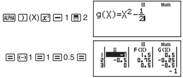
**Note:** • The maximum number of rows in the generated number table depends on the setup menu table setting. Up to 30 rows are supported for the "f(x)"
