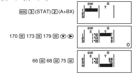
**Important:** • All data currently input in the Stat Editor is deleted whenever you exit the STAT Mode, switch between the single-variable and a paired-variable statistical calculation type, or change the Stat Format setting on the setup menu. • The following operations are not supported by the Stat Editor:  $\mathbb{M}$ ,  $\mathbb{H}$ , \mathbb
