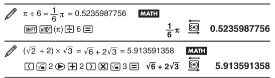
While Linear Display is selected, each press of Em will toggle the currently displayed calculation result between its decimal form and fraction form.
