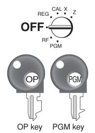
The position of the Mode Switch controls the type of operations you can perform on the cash register. The PROGRAM key (marked PGM) can be select any Mode Switch setting, while OPERATOR key (marked OP) can be used to select OFF, REG or CAL only.
