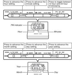
Slide the **Mode switch** (§) to "NORMAL". This will cause the figures on the display to stop flashing.
