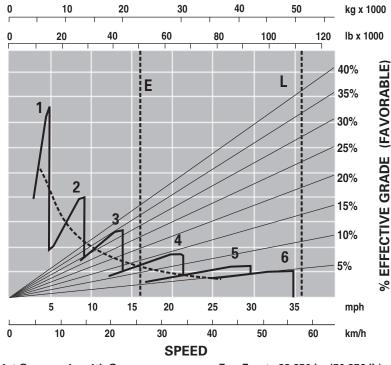
1 — 1st Gear 4 — 4th Gear 2 — 2nd Gear 5 — 5th Gear 3 — 3rd Gear 6 — 6th Gear
