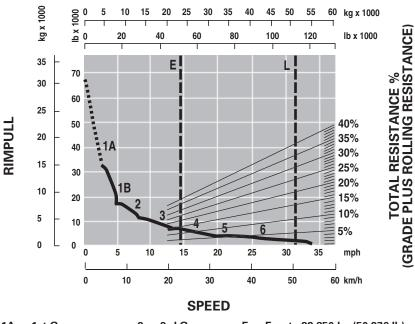
1A — 1st Gear 3 — 3rd Gear (Converter Drive) 4 — 4th Gear 1B — 1st Gear 5 — 5th Gear (Direct Drive) 6 — 6th Gear
