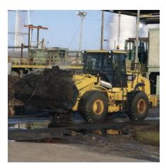
**Woodchip and Clean-Up Buckets.** Woodchip and high-capacity clean-up buckets are available for forestry and millyard applications.
