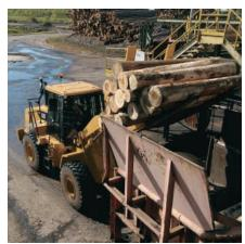
**LOAD SENSING HYDRAULICS.** The 950H features a load sensing hydraulic system that automatically adjusts to operating conditions to provide only the hydraulic flow required by the implement for improved fuel efficiency.
