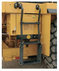
**ENTRY AND EXIT.** A ladder with selfcleaning steps keeps debris build-up to a minimum. The ladder is at a  $5^{\circ}$ forward incline for easy entry and exit.
