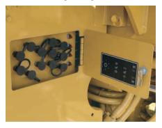
**REMOTE PRESSURE TAPS.** Pressure taps for the steering and hydraulic systems, transmission (optional) and brakes are grouped behind an access panel just below the right-side service platform.
