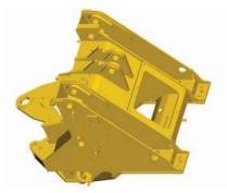
**Non-Engine End Frame (NEEF).** The non-engine end frame provides a solid mounting base for the front axle, lift arms, lift cylinders and tilt cylinders. The fabricated, four-plate loader tower absorbs the forces associated with loading, twisting and penetration.
