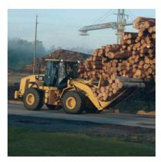
**RIDE CONTROL.** The optional Ride Control System improves ride, performance and load retention when traveling over rough terrain. Operators gain confidence moving at higher speeds in load and carry operations decreasing cycle times and increasing productivity.
