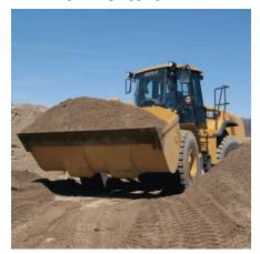
**POWERSHIFT TRANSMISSION**. The 950H continues to use heavy-duty powershift transmission technology proven on previous models and currently used up through the largest wheel loader built by Caterpillar - the 994F.
