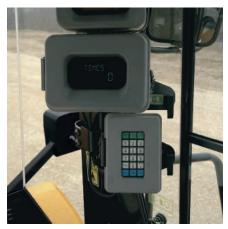
**PAYLOAD CONTROL SYSTEM.** Scales, designed specifically for Cat machines allow on-the-go weighing of material in the bucket. Operators load trucks more accurately and efficiently. Loading trucks right the first time equates to quicker cycles for the operator and more productivity and controllability for your operation.
