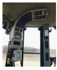
**CONTROLS.** The main control panel on the 950H is located high on the right ROPS post - keeping everything within reach of the operator while maintaining visibility to the ground. Keeping all switches and controls conveniently placed allows better efficiency and improved productivity all while minimizing operator fatigue.
