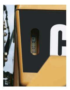
**SIGHT GAUGES.** Well-protected, yet easily visible sight gauges for the transmission, hydraulic oil and radiator coolant allow easy daily checks while reducing the risk of contaminants entering the systems.
