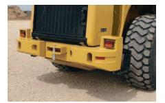
**Counterweight.** The two-piece counterweight is integrated into the 950H design and styling. This 1853 lb (840 kg) counterweight incorporates the rear lights into the top of the structure.
