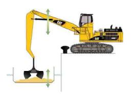
**Material Handling.** It is more efficient and productive due to faster return cycles. Unloading barges is easier because SmartBoom avoids excessive force being put on the floor of the barge allowing the operator to fully concentrate on production.
