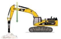
Hammer Work. It has never been this productive and operator-friendly. The front parts automatically follow the hammer while penetrating the rock. Blank shots or excessive force on the hammer are avoided resulting in longer life for the hammer and the machine. Similar advantages are applicable when using vibratory plates.
