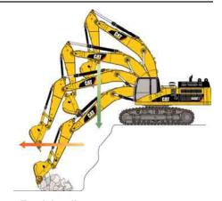
**Truck Loading.** Loading trucks from a bench is more productive and more fuel efficient as the return cycle is reduced while the boom down function does not require pump flow.
