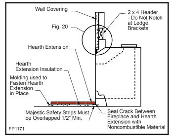
Fig. 30 Sealing detail.
