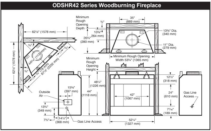
Fig. 1 ODSHR42 Series specifications and framing.
