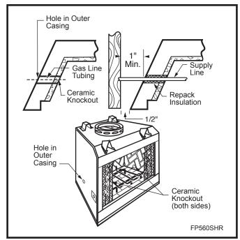
Fig. 32 Gas line access.
