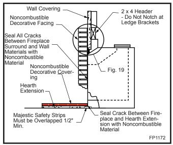
Fig. 31 Sealing detail.
