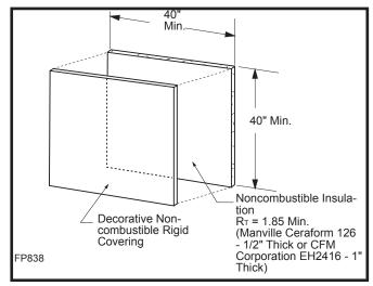
Fig. 26 Noncombustible wall shield dimensions.
