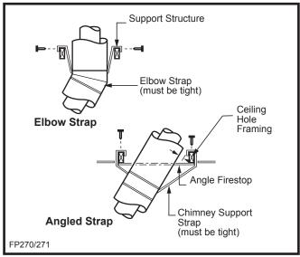
Fig. 18 Attach straps to a structural framing member.
