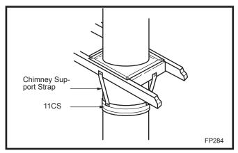
Fig. 9 Chimney support installation
