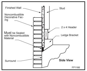
Fig. 21 Fireplace surround flush with finished wall.
