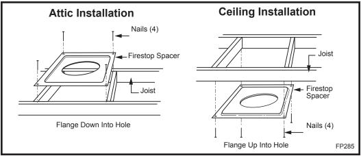
Fig. 19 Installing firestop spacer.
