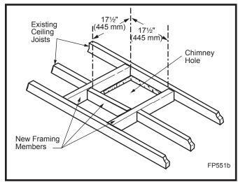
Fig. 13 Typical frame for ceiling chimney hole.
