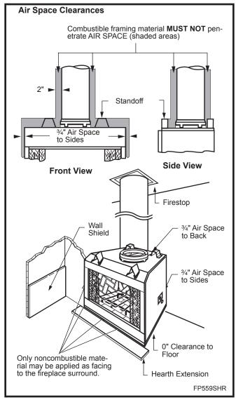
Fig. 20 Minimum clearances to combustibles.
