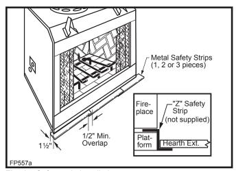
Fig. 14 Safety strip installation.
