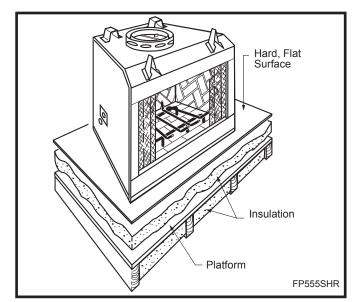
Fig. 10 Insulating between platform and fireplace.
