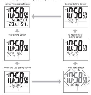
2. While the screen you want is displayed, use the - (DOWN) and + (UP) buttons (4) to change the flashing digits.
